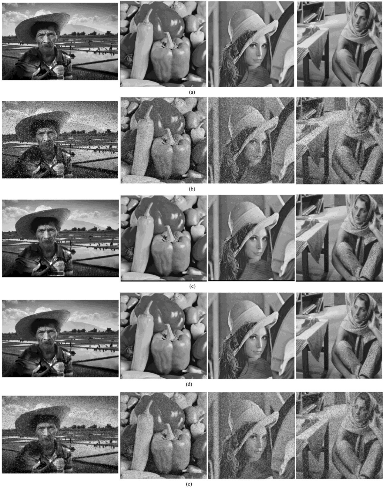
Fig. 12. (a) Original images; (b) noisy images by 10% and 20% salt and pepper noise for the left and right images respectively; (c) images denoised by the proposed method; (d) images denoised by median filter in MATLAB software; (e) image de-noising by mean filter in MATLAB software.
