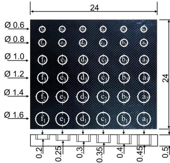
Fig. 2 CFRP specimen layout (dimensions in cm)
