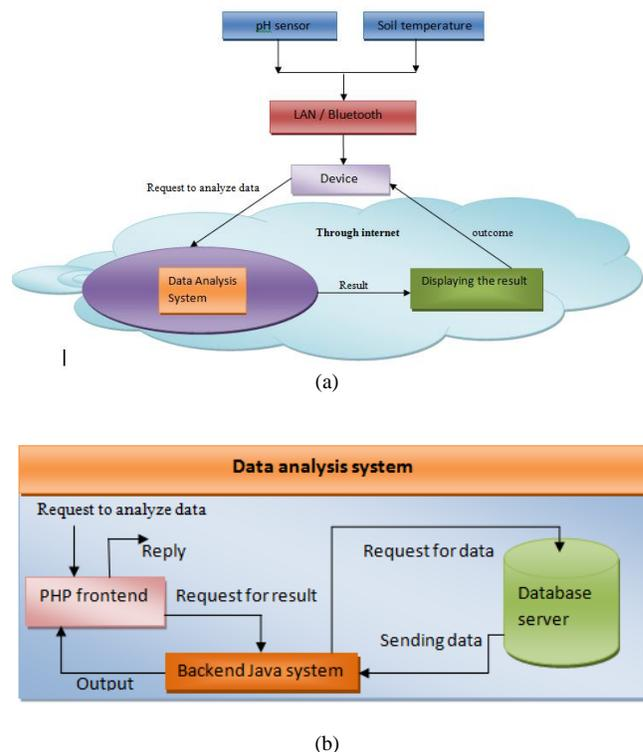
Fig. 1 (a) Schematic of system structure, (b) Data analysis system.
