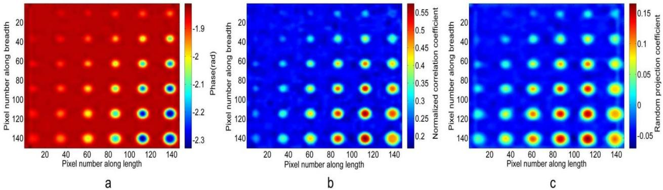
Fig. 4 Processed results of CFRP sample for QFMTWI a. FFT phase at 0.05Hz, b. Correlation image at 7.8s and c. Random projection image at 4<sup>th</sup> component
