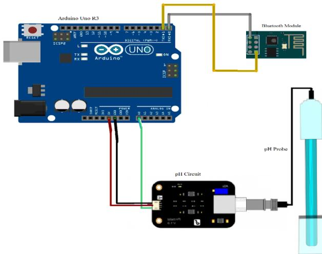
Fig. 3 Circuit diagram of the hardware units.
