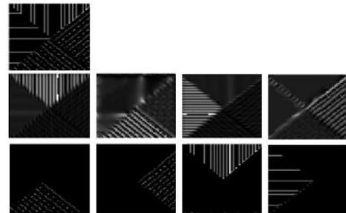
Fig 7: Output of Gabor filter in four directions when input of an image contains lines in similar frequencies but in different angles [16].
