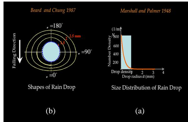
Fig 2: Distribution Marshall - Palmer count raindrops, as a function of their size. Figure (a) Note that the density drops exponentially with the size of the rain falls. Image (b) is the shape of raindrops of different sizes (0.5 to 2.5 mm). Due to the drop in flat form (an oblate spheroid shape) are falling [15].
