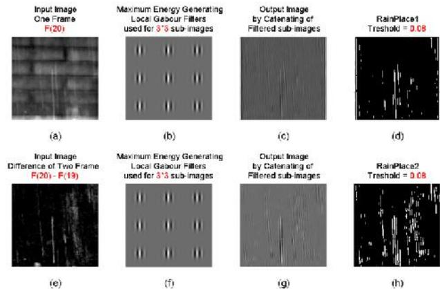
Fig 12: Rain detection of each frame using background subtraction and dominant direction of Gabor filter (3\*3). Figures (a) to (d) relate to frame 20 of main video, Gabor filters with dominant directions, filtered image and rain place after thresholding, respectively. Other explanations are similar to Figure (11).
