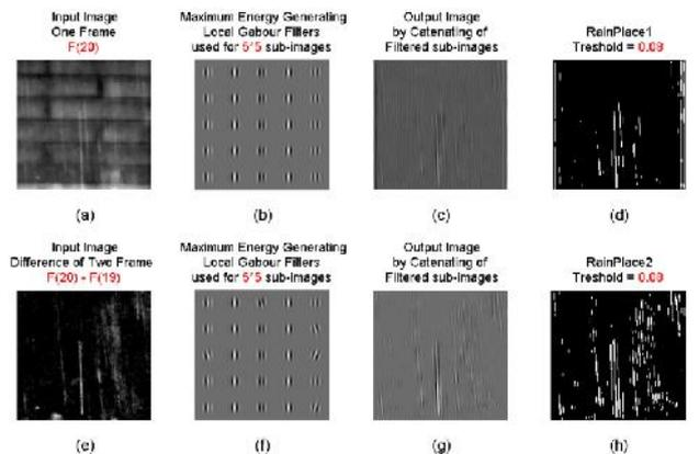
Fig 14: Rain detection of each frame using background subtraction and dominant direction of Gabor filter (5\*5). Figures (a) to (d) relate to frame 20 of main video, Gabor filters with dominant directions, filtered image and rain place after thresholding, respectively. Other explanations are similar to Figure (11).
