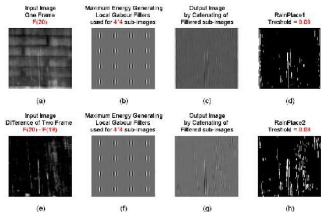
Fig 13: Rain detection of each frame using background subtraction and dominant direction of Gabor filter (4\*4). Figures (a) to (d) relate to frame 20 of main video, Gabor filters with dominant directions, filtered image and rain place after thresholding, respectively. Other explanations are similar to Figure (11).
