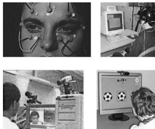
Fig. 1: Two samples of systems used in intrusive (top row) and non-intrusive (bottom row) methods [7, 17].
