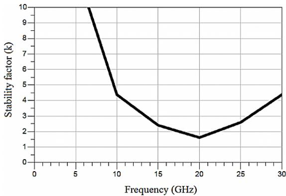
Fig. 8. Simulated stability factor (k) of the proposed CMOS-DA
