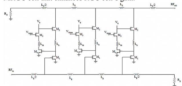
Fig. 2. The circuit topology of the proposed CMOS-DA
